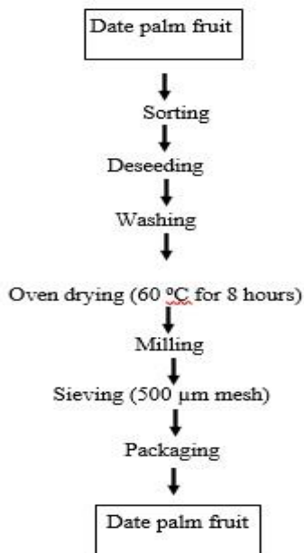
Figure 3: Flow chart for date palm fruit flour production.
