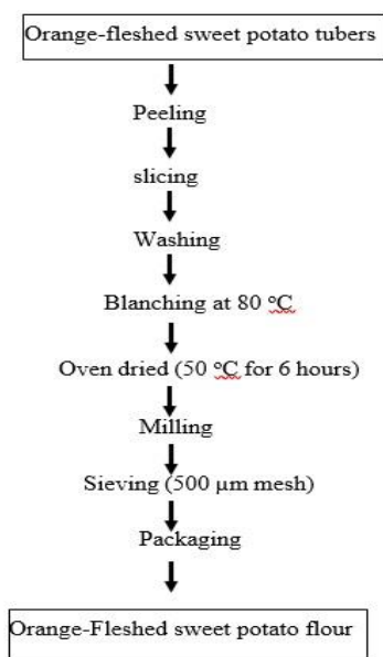
Figure 1: Orange-Fleshed sweet potato flour Production
