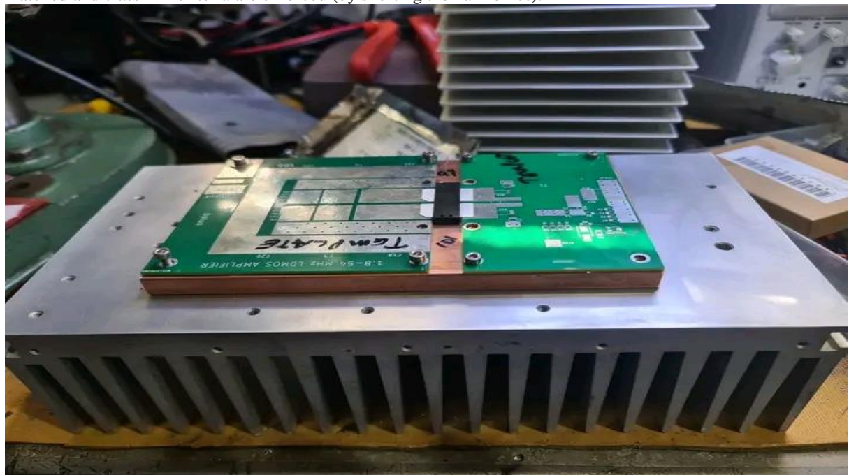
Figure 14. Construction of RF LDMOS
