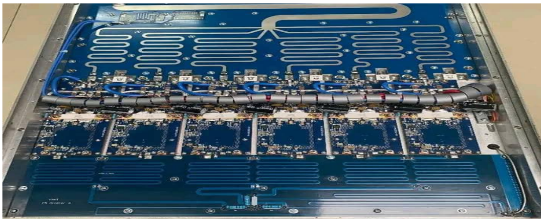
Figure 8. Photograph of combined amplification using Strip lines
