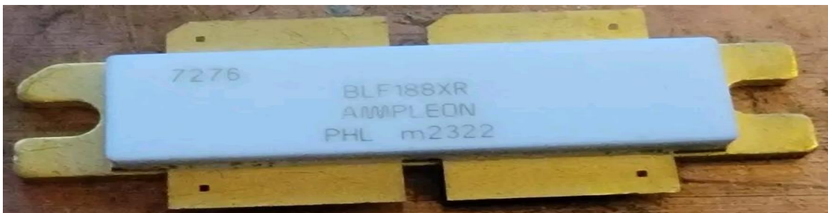
Figure 5. Photograph of BLF188XR MOSFET
