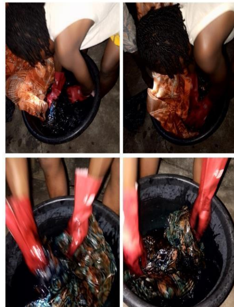
Plate 34: Dyeing the already waxed fabric Source: Nwankwo (2024)
