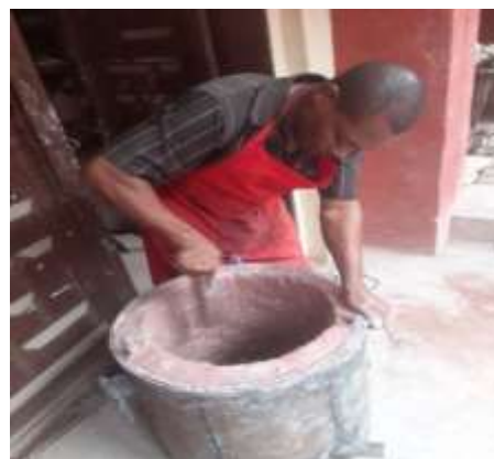
Plate 15: The Researcher Filling and Ramming Clay upon Fiberglass Lining in the Combustion Chamber. Source: Photograph taken by Gaius.
