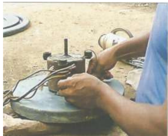
Plate 11: The researcher fixing the Blower on the Casing. Source: Pix taken by Gaius Ikenna.
