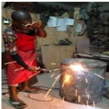
Plate 6; Shows How Top of the Cover was Welded on Shell Before Cutting. Source: Photograph taken by Gaius.
