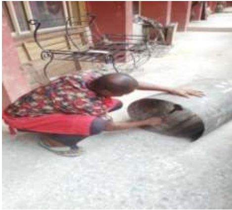
Plate 3: Showing the Researcher Hammering the Rolled Sheet Metal Source: Phot by Gaius.
