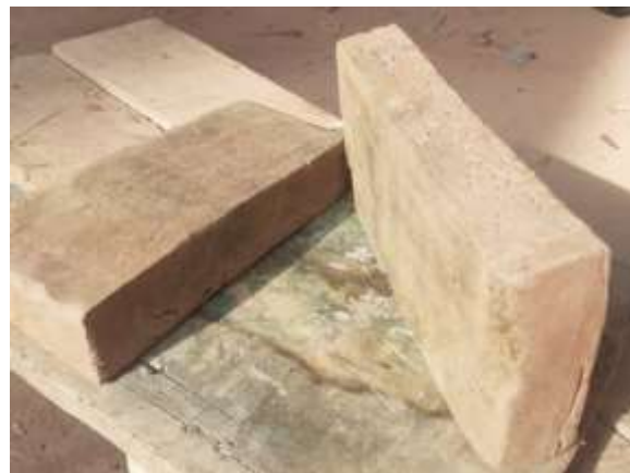
Plate 13: Sample of the Brick used in the Combustion Chamber. Source: Photo by the Researcher.
