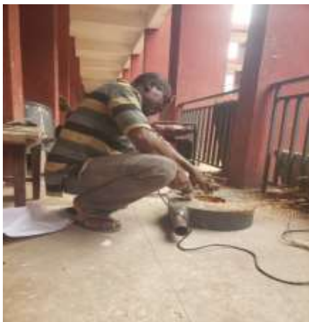
Plate 10: The Sculptor Cutting Open a Void for Air Draft-in the Box. Source: Photograph taken by Gaius Ikenna.
