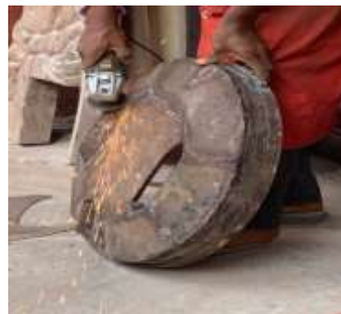
Plate 7: The Researcher is Shown Cutting Open Spaces for the Vents Source: Photo by Gaius
